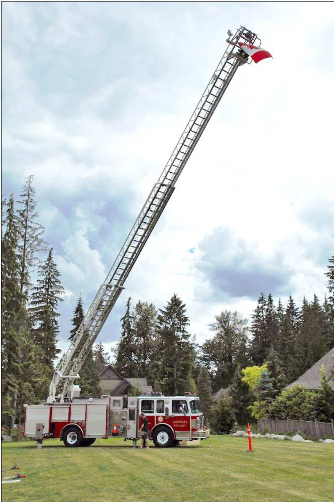
SVFD's Ladder Truck #7 — 75-Foot Ladder Fully Extended
